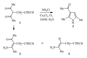
The greatest yield of pyrrole 2 (49%) was achieved using a three-fold excess of  $Cu_2Cl_2$  and 10-fold excess of NH<sub>4</sub>Cl. Pyrrole 2, whose structure was confirmed by elemental analysis, IR and <sup>1</sup>H NMR spectroscopy, is a rather stable compound, which darkens upon exposure to light. This compound may be stored for a long period in a refrigerator in the dark but undergoes partial decomposition to an enamine and the starting ketone upon chromatography on silica gel.
